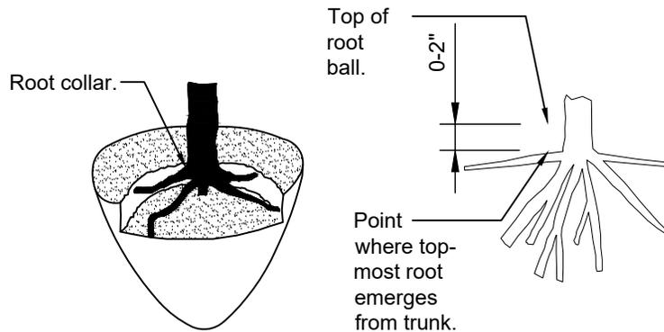
The point where top-most root(s) emerges from the trunk (root collar) should be within the top 2" of substrate. The root collar and the root ball interior should be free of defects including circling, kinked, ascending, and stem girdling roots. Structural roots shall reach the periphery near the top of the root ball.
