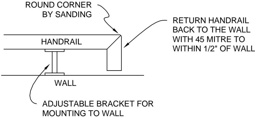
HANDRAIL TO BE FABRICATED FROM RED OAK WITH CLEAR FINISH
