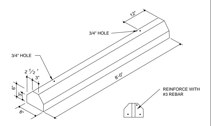
2'-4'-6'-8' Standard lengths 3'-5'-7' Special order lengths Concrete: 3500 P.S.I. at 28 days Weight: 38lbs per linear foot 5/8" x 12" pins to fasten to pavement
