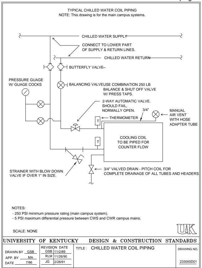
233000D01 HVAC AIR DIST. Chilled Water Coil Piping
