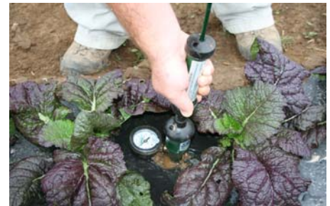
Making a hole with a soil probe, filling with water to form a slurry, and pulling suction on the inserted tensiometer make for a tight seal and accurate measurements.
