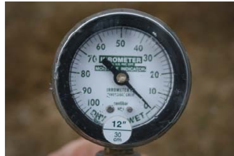
(Left) Tensiometers ranging in size from six to eighteen inches, (Right) the vacuum gauge on a tensiometer reads in units of centibars
