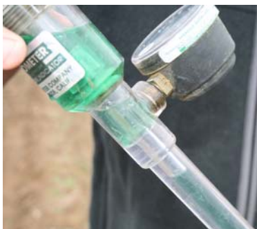
Tensiometers will not read accurately when air gaps are present.
