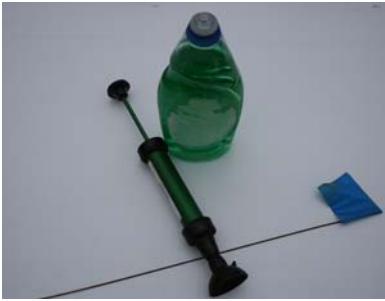
Tools for tensiometer preparation: Water with dye, suction device, and field flag
