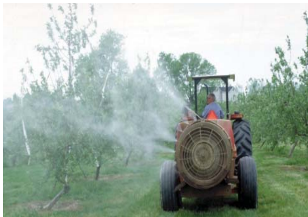
Figure 2. Apple orchard air blast sprayer used for applying fungicides for scab control.
